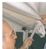
The frame's adjusters are tightened and the loose hanging sun canopy is tightened to the trailer body canvas by using the ribbons.
